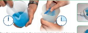
Pour the components in the measuring beaker, mix and leave to cross link (about 15 minutes). Remove the insulation and position it in small parts around the connection so that it is fully covered. Insulation saved from previous mixes can of course be utilised.
