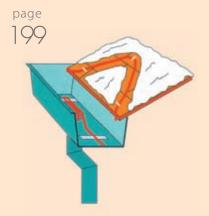
MCA8 Self-regulating cable for tracking roofs, gutters and/or downpipes
