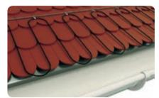
Power: 20 W/m **Power supply:** 230 V ~ 50/60 Hz Heating cable dimensions:  $\sim 5 \times 7 \text{ mm}$ Min. installation temperature:  $+5^{\circ}$ C Max. working temperature: +80°C Cold cable (power supply): length 4 meters - 3 x 1,0 mm<sup>2</sup> or 3 x 1,5 mm<sup>2</sup>
