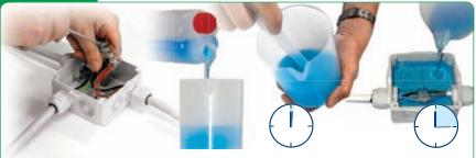
You can use the Magic Power gel supplied in the bicomponent bottle in a 1:1 ratio by simply pouring it after mixing into the box supplied in the kit, to protect and seal internal connections. The gel cross links in just 15 minutes, but the box can be energised immediately.
